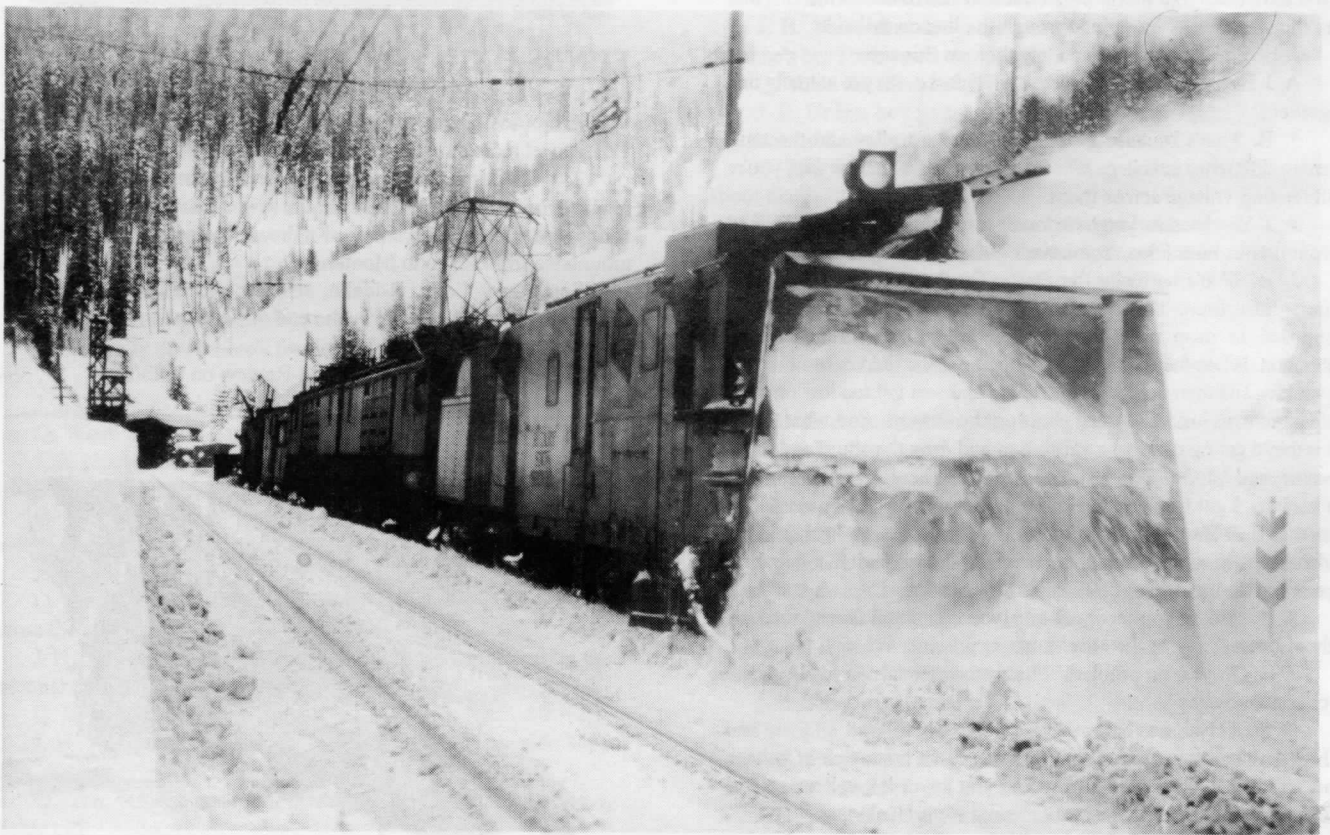
Steam rotary plow at East Portal, MT 1930's. The plow is clearing the siding.
